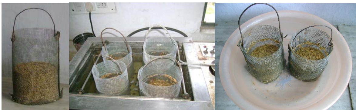
Figure 1 The laboratory arrangement for soaking experiments
